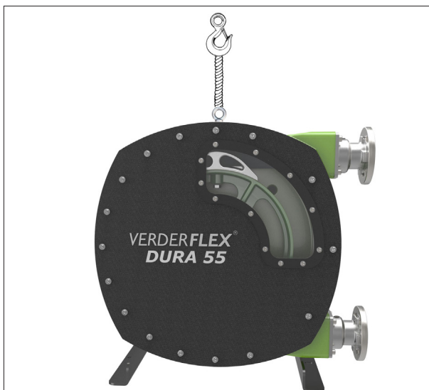
Figure 1. - Fastening lifting gear to pump
