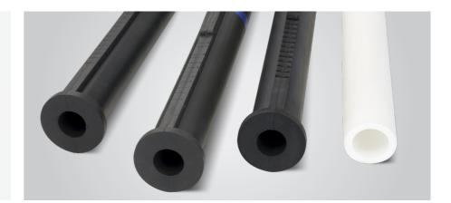
The CSM or Hypalon<sup>®</sup> hose is used when highly corrosive media, e.g. strongly oxidizing media, must be transferred. The inner layer is made of CSM, the outer surface of SBR / NR. Hypalon is a trademark of
